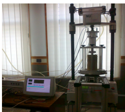
Fig 6: Resilient Modulus test in progress
